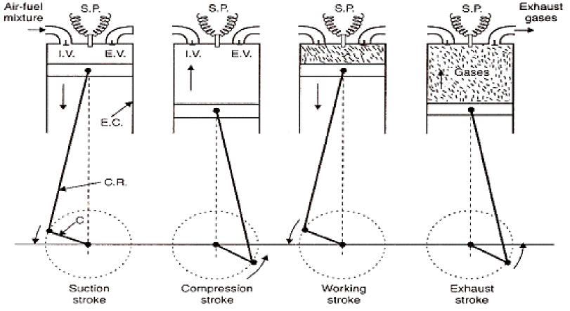
I.V = Intel valve, E.V. = Exhaust valve, E.C. = Engine cylinder, C.R. = Connecting rod C = Crank, S.P. = Spark plug.
