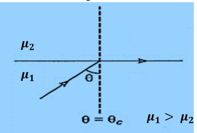
c) When the angle of incidence is further increased ( $\theta > \theta_c$ ), the ray is reflected back in the same medium. This phenomenon is called as **total internal reflection**.
