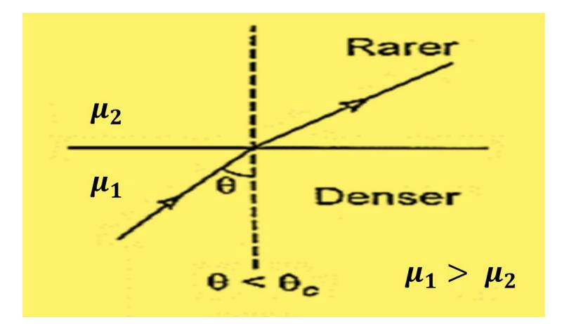
**b**) For a particular angle of incidence, the refracted ray just grazes the interface between the two media as shown in figure. This angle of incidence is called critical angle.
