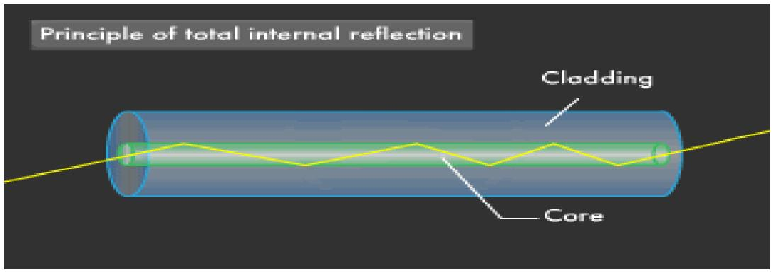
With the help of well labeled diagram, name the components of an optical fibre. [2015-16, 2020-21]
