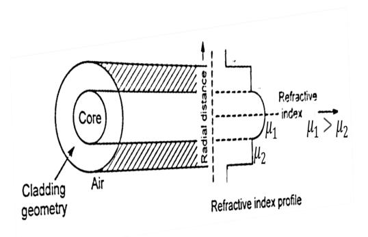
The light rays propagate through it in the form of skew rays or helical rays. They do not cross the fibre axis at any time and are propagating around the fibre axis in helical or spiral manner.
