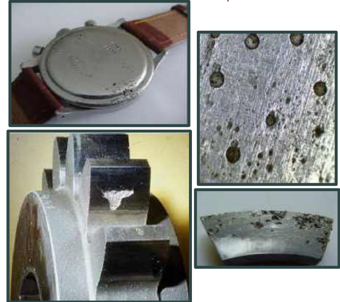
Images to show Pitting corrosion
