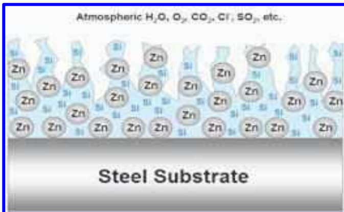
Inorganic coating to prevent corrosion
