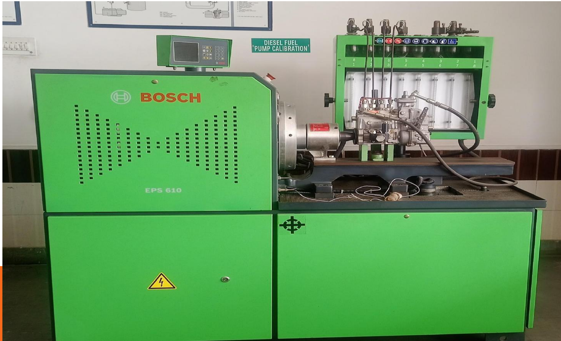
DIESEL FUEL PUMP CALIBRATION MACHINE
