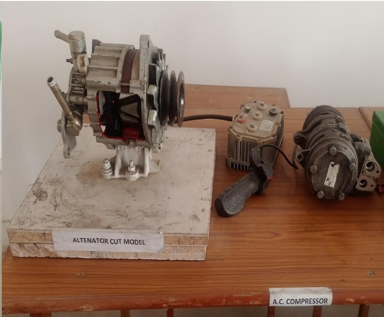
ALTERNATOR CUT MODEL & AC COMPRESSOR
